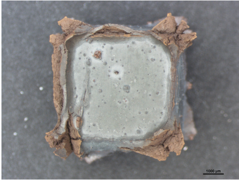
Figure 44: An oxidized W-10%Cr-2%Ti alloy at 1273 K. Oxidized structures appeared at the edges of the sample.
