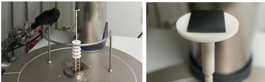
(a) The TGA system with opened chamber. The sample holder and an oxidized tungsten sample on top of the sample holder are shown.
