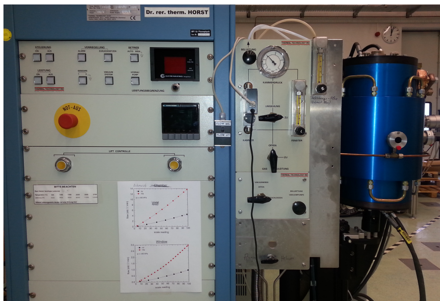
Figure 14: Oven called "HORST". The machine is used to heat up the sample at approximately 2100 K for 35 min.
