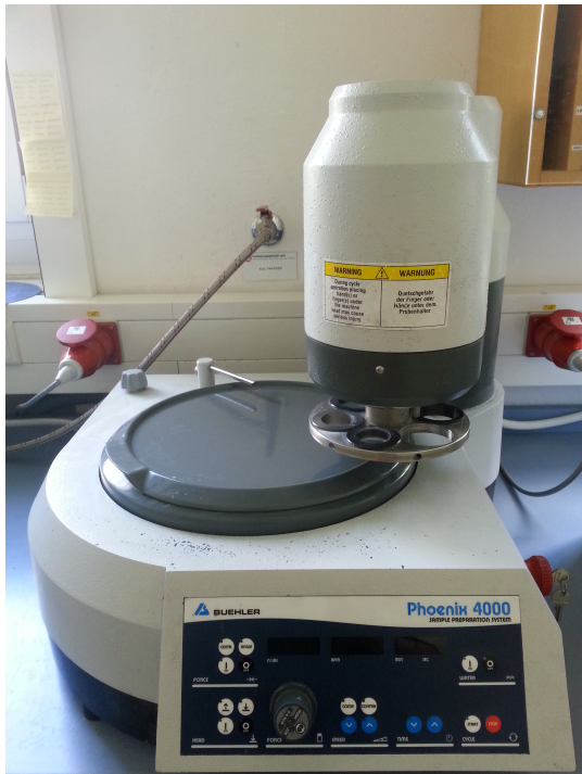
(a) "Phoenix 4000" grinding machine.
