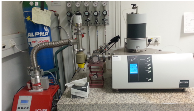
(a) The TGA system and the vacuum system used in the laboratory.
