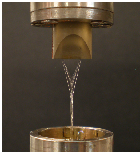
Figure 4.2: The sapphire nozzle produces a liquid flat sheet jet of 100 \mu\text{m} thickness over a width of about 6 mm. The sheet flows downwards at an adjustable speed in the range of 0.5 m/s to 30 m/s (in this photo: \sim 5 m/s).
