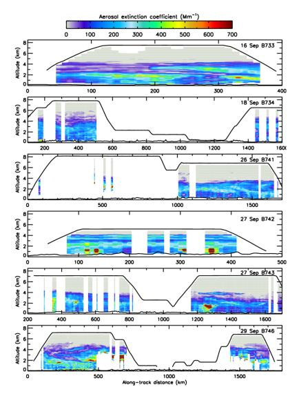
**Figure 10.** Cross sections of the aerosol extinction at 355 nm coefficient determined from the lidar for the six research flights with a 1 min integration time. The black lines indicate the aircraft altitude and the surface elevation from a digital elevation model, respectively.
