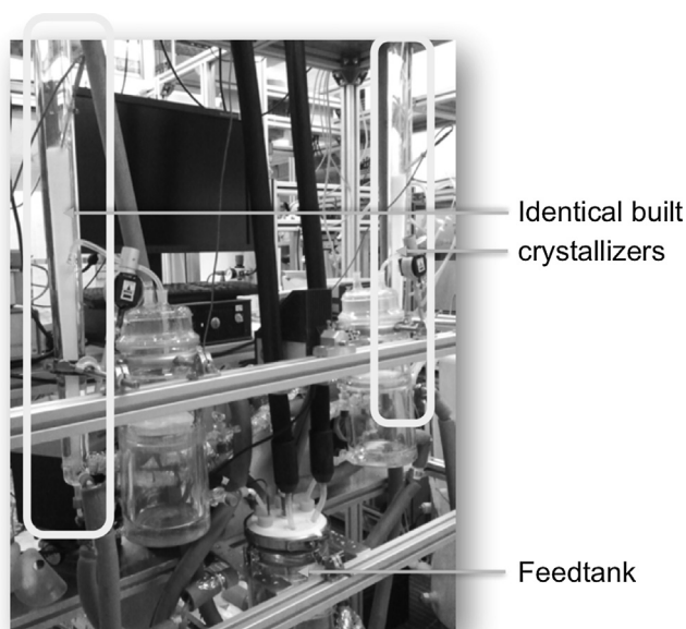
Fig. 2. Existing test apparatus installed at MPI Magdeburg.
