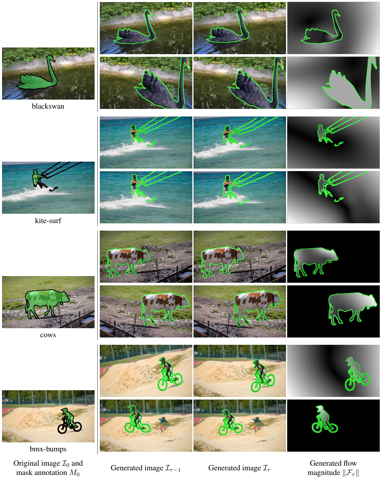
Figure S1: Lucid data dreaming examples. From one annotated frame we generate pairs of images (\mathcal{I}_{\tau-1}, \mathcal{I}_\tau) that are plausible future video frames, with known optical flow (\mathcal{F}_\tau) and masks (green boundaries). Note the inpainted background and foreground/background deformations.
