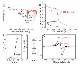
**Fig. 2** (a) FT-IR spectrum of B-BT, (b) diffuse reflectance (DR) UV/Vis spectra of pure and B-BT-coated glass fibers, (c) Kubelka–Munk-transformed reflectance spectrum of B-BT, (d) HOMO and LUMO positions of B-BT, and (e) EPR spectra of B-BT in the dark and under visible light irradiation.
