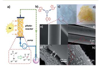
Fig. 1 (a) An illustrated setup of a fixed-bed photoreactor using conjugated nanoporous polymer-coated glass fibers. (b) Molecular structure of B-BT. (c) Photography of pure glass fibers and (d) B-BT-coated glass fibers. (e) SEM images of pure glass fibers and (f-h) B-BT-coated glass fibers.
