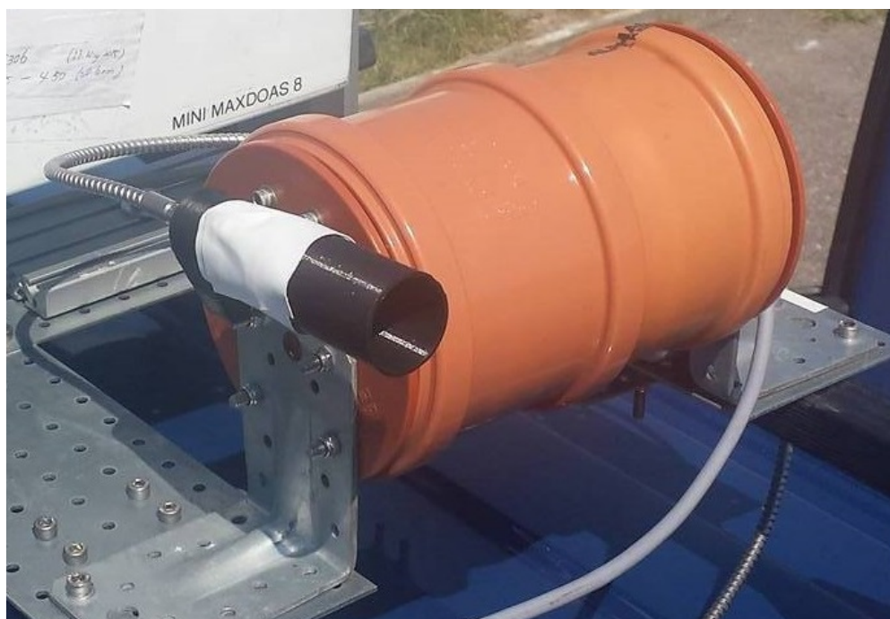
Figure 4.2.: On-roof unit of the TubeMAX-DOAS instrument. The orange tube contains the motor which moves the telescope.
