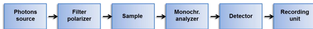
Fig. 2.3 – 5 General set-up for the recording of luminescence spectra with a photon excitation source.
