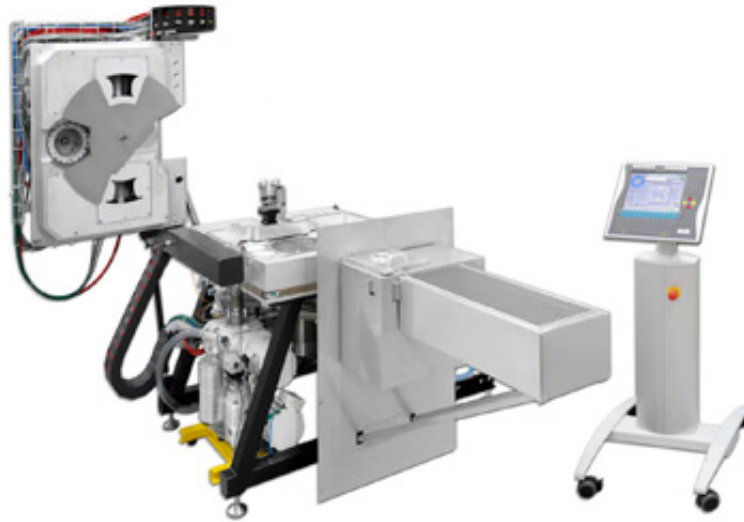
Figure 3.2: The Helios magnetron sputtering system of LEYBOLD OPTICS (BÜHLER AG) integrates the intermittent deposition technique in a chamber that is never opened to atmosphere except when servicing is necessary. Figure adapted from [56].
