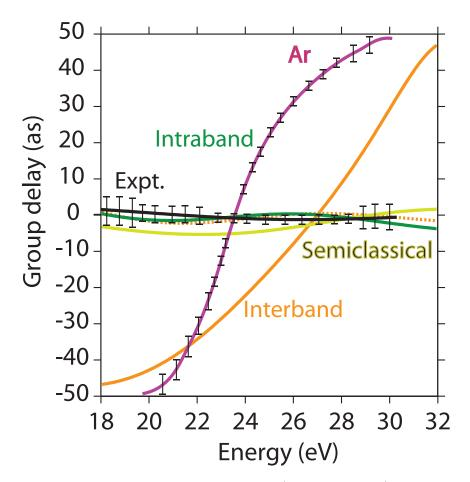
Figure 4.14: Experimentally retrieved group delays (emission times) of a single attosecond burst from  $SiO_2$  (black line) and a single attosecond burst from Ar gas (violet line) in addition to the theoretical values for the interband polarization (orange line), the intraband current (green line), total polarization (orange dashed curve) and the semiclassical model (yellow line).
