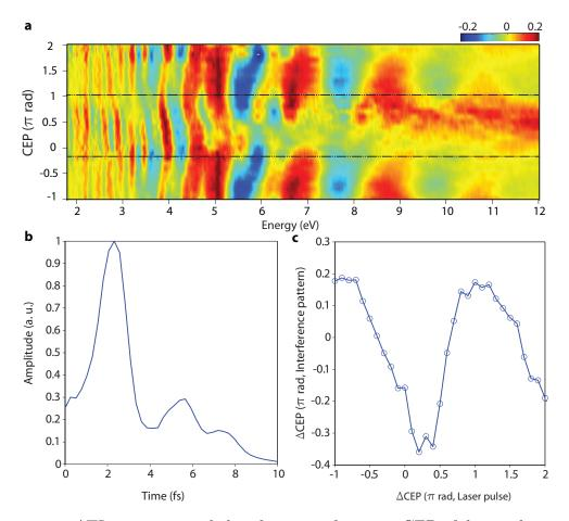
Figure 5.11: **a**, ATI spectra recorded as function of varying CEP of driving laser pulse. **b**, FT of one of the measured spectra. **c**, CEP variation of the ATI pulse train as a function of the varying CEP of driving laser pulse.
