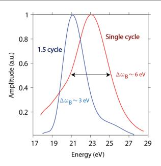
Figure 4.24: Retrieved EUV spectrum from attosecond streaking measurements performed with a single cycle driver (red curve) and a one and half cycle driver pulses in  $SiO_2$ .
