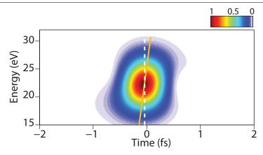
Figure 4.4: Time-frequency spectrogram of the retrieved EUV attosecond pulse from the measured streaking spectrogram shown in Figure 4.3. Solid orange curve is tilted and white dashed curve is vertical to connote for positive chirp of EUV emission.
