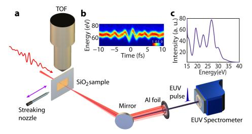
Figure 3.1: **a**, Experimental set-up used for measuring HH EUV emission from SiO<sub>2</sub> nanofilms (thickness ~ 120*nm*). **b**, Attosecond streaking spectrogram recorded to retrieve the optical field waveform before being focused on SiO<sub>2</sub>. **c**, A typical EUV spectrum measured by a 1.5 cycle driving optical waveform.
