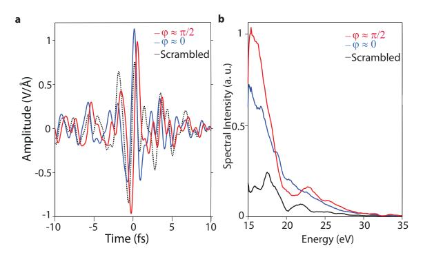
Figure 3.5: Spectral control over EUV emission steered by sculpted light waveforms: **a**, optical attosecond pulse; red curve - CEP = 0 rad; blue curve - CEP =  $\pi/2$ rad and a scrambled waveform (black dashed curve). **b**, EUV spectra generated by optical waveforms shown in **a**.
