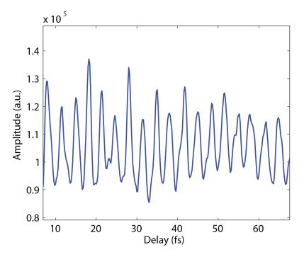
Figure 7.4: Temporal modulation of spectral intensity of resonant line at 8.43 eV as a function of delay between pump and probe optical attosecond pulses.
