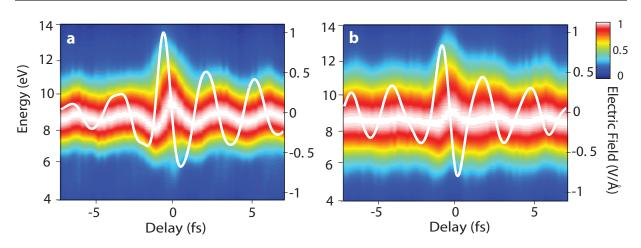
Figure 4.20: **a**, **b**, Attosecond streaking spectrograms recorded for two CEP settings of the single-cycle driver waveform (white lines on top of spectrograms), differing by  $\pi/2$  rad.
