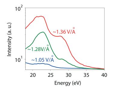
Figure 3.8: Cut-off scaling of EUV emission continua to more than 35 eV by driving  $SiO_2$  nanonfilms with increasing field strengths of an optical attosecond pulse.
