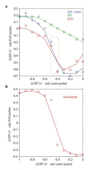
Figure 5.12: **a**, Alteration of CEP of ATI pulse train, EUV attosecond pulse and ATI-EUV interference pattern on CEP variation of the driving laser pulse, displayed orange rectangular box shows the swift jump of CEP of EUV pulse around 0.5  $\pi$  rad CEP of driving pulse. **b**, CEP variation of isolated EUV attosecond pulse as calculated by semicalssical model.
