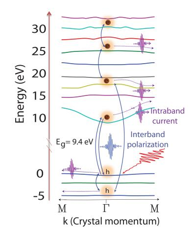
Figure 4.11: Interband Vs Intraband dynamics behind EUV emission from  $SiO_2$ . Multilevel Quantum mechanical model for simulating EUV emission, optical driver pulses couple electrons and holes in the valence and conduction bands which are then driven in opposite directions. Electron-hole motion along the bands gives rise to intraband current whereas the dipole arising out of dynamic excitation-relaxation between the bands during interaction with the field gives rise to interband polarization.
