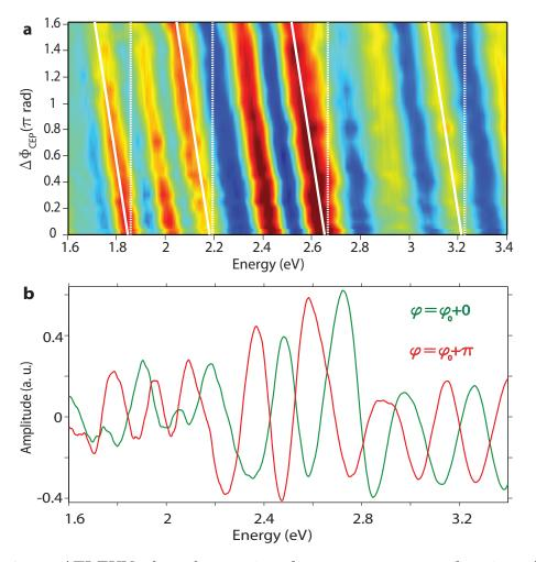
Figure 5.3: **a**, ATI-EUV photoelectron interference spectra as a function of the CEP variation of EUV pulse, solid white (tilted) and white dashed (vertical) lines are to guide the eyes to the linear variation of interference pattern on linear variation of CEP of EUV pulses. **b**, Comparison of spectral interference pattern for two different CEPs of EUV pulse differing by  $\Delta \phi_{CEP} \approx \pi$  rad.
