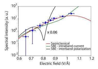
Figure 3.3: Spectral amplitude scaling of  $11^{th}$  harmonic as measured in our experiment compared to that simulated from semi-classical and Quantum-mechanical simulations. This figure has been adapted from [23].
