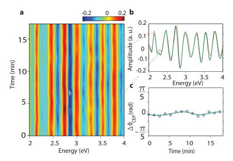
Figure 5.8: **a**, Spectral interference between ATI and EUV photoelectrons in Ar recorded for more than 15 minutes. **b**, comparison of spectral interference pattern recorded at two different moments of time. **c**, Evaluated CEP of EUV pulses (intraband current) as retrieved from spectra in **a**.
