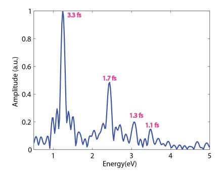
Figure 7.5: Observed frequencies of quantum interferences arising from coherent coupling of state at 8.43 eV with other excited states.
