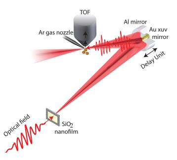
Figure 4.8: **Delay synchronization experimental set-up**. Optical driving laser pulses are reflected-off the dual mirror assembly and focused on an Ar gas jet, low energy electrons generated by highly nonlinear processes (e.g. direct or rescattered electrons in above threshold ionization) are detected in TOF.
