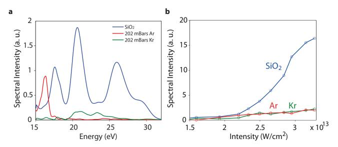
Figure 3.6: **a**, Comparison of spectra emitted by identical number of emitters in SiO<sub>2</sub>, Ar and Kr with intensity of driving optical pulse being  $2X10^{13}W/cm^2$ . **b**, Comparison of spectral flux scaling of SiO<sub>2</sub> with Ar and Kr under similar experimental conditions.
