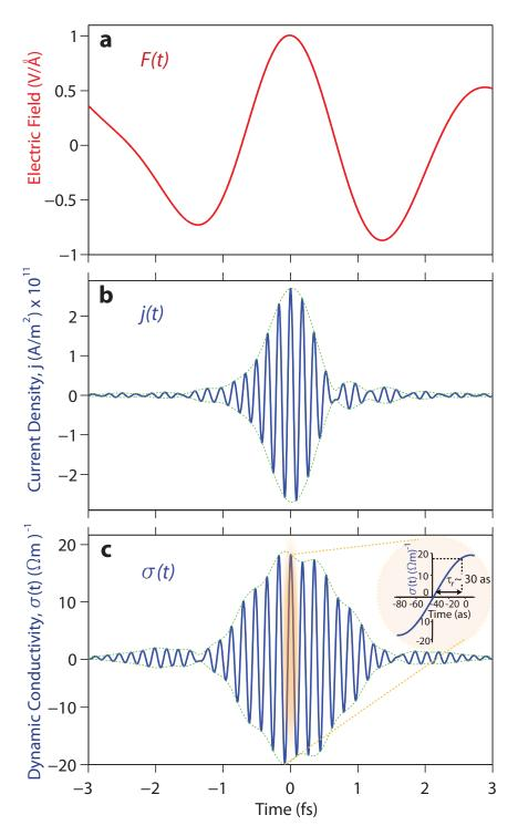
Figure 4.28: Nonlinear multi-PHz current density and dynamic conductivity of SiO<sub>2</sub>. **a**, Temporal profile of the optical field generating nonlinear intraband electric current in SiO<sub>2</sub>. **b**, **c**, Evaluated nonlinear current density j(t) and dynamic conductivity  $\sigma(t)$  in SiO<sub>2</sub> respectively. Inset in Figure 4.28c highlights the rapid switching of the conductivity within approximately ~ 30 as.
