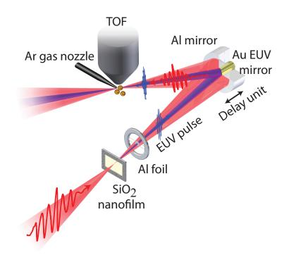
Figure 4.1: Experimental setup. The radiation emanating from SiO<sub>2</sub> nanofilms (~ 120nm) was spectrally filtered (> 15 eV) and spatially separated from the light waveform generating EUV radiation. Both beams were temporally delayed with respect to each other and were focused on an Ar gas target by a two-component concentric mirror assembly. The photoelectron spectra were recorded by a time-of-flight (TOF) spectrometer as a function of the time delay between the two pulses.
