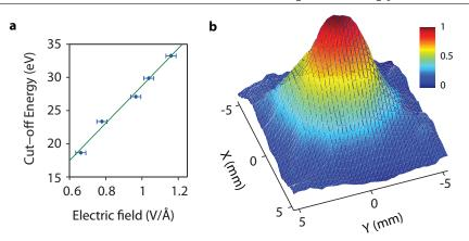
Figure 3.2: **a**, Scaling of cut-off energy with the driving field strength of EUV emission measured with a 1.5 cycle driving waveform. **b**, Far-field spatial intensity profile of EUV emission measured with an image intensifier. This figure has been adapted from [23].
