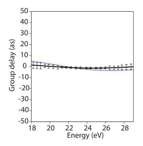
Figure C.3: Group delay of EUV pulses generated from  $SiO_2$  as retrieved from experiments (blue dashed curve) and the group delay after accounting for spectral phase correction from the measurement set-up (solid black curve).
