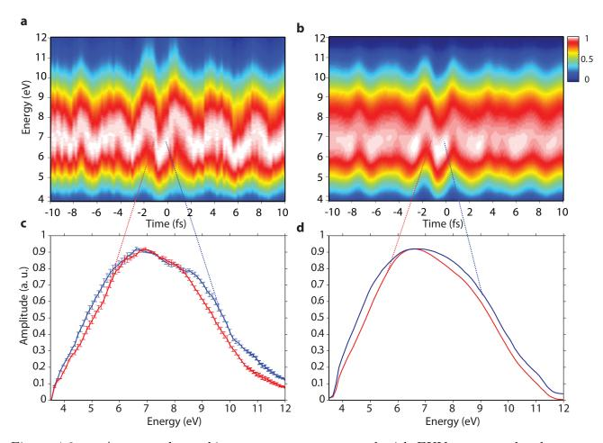
Figure 4.6: **a**, Attosecond streaking spectrogram measured with EUV attosecond pulses generated in Ar.**b**, Reconstructed spectrogram of measurement in **a** by PCGPA. **c**, **d** Representative spectra sampled at zero-crossings of the vector potential around the peak of the streaking field provide direct evidence of the positively chirped EUV dynamics. Error bars on experimental spectra are the standard error derived from consecutive measurements under identical conditions.
