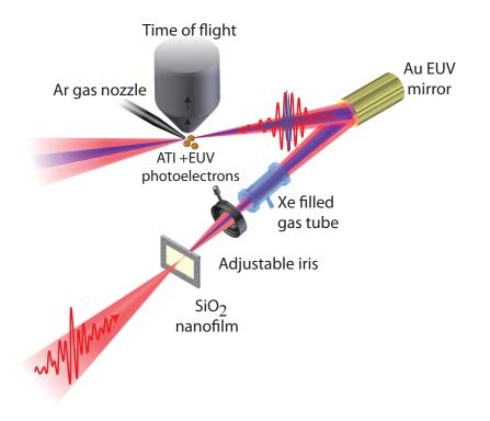
Figure 5.1: Experimental set-up: EUV pulses generated from a  $SiO_2$  nanofilm and the optical driver are reflected-off an Au coated mirror and focused onto an Ar gas jet. Photoelectrons generated by ATI and direct photoionization by EUV pulses are recorded in TOF spectrometer. Variation of Xe gas pressure in a gas tube along the beam path of EUV pulse introduces a definite amount of CEP variation on EUV pulse.
