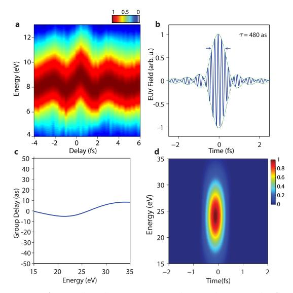
Figure 4.19: **a**, Attosecond streaking measurement with EUV pulses generated in Quartz (thickness ~ 5  $\mu$ m) **b**, Retrieved isolated attosecond pulse after the convergence of PCGPA. **c**, Retrieved group delay (emission time) of the single EUV attosecond burst. **d**, Time-frequency spectrogram of the retrieved attosecond pulse.
