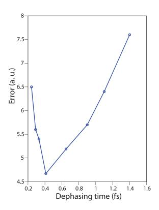
Figure 6.3: Variation of difference (error) between experimentally recorded spectrogram (Figure 6.1a) and the spectrograms simulated by SBEs for different dephasing times, a minima in the error at  $\sim 400$  as dephasing time for interband polarization connote to best agreement between the simulation and the experiment.
