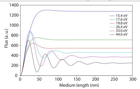
Figure 3.7: Phase matching considerations of EUV generation in SiO<sub>2</sub>. Buildup of EUV flux versus propagation length calculated for representative photon energies (mentioned in the legend). Material parameters are taken from Ref. [68]. Comparable results (within 10% accuracy) can also be obtained based on data from Ref. [69] for photons higher than 30 eV.
