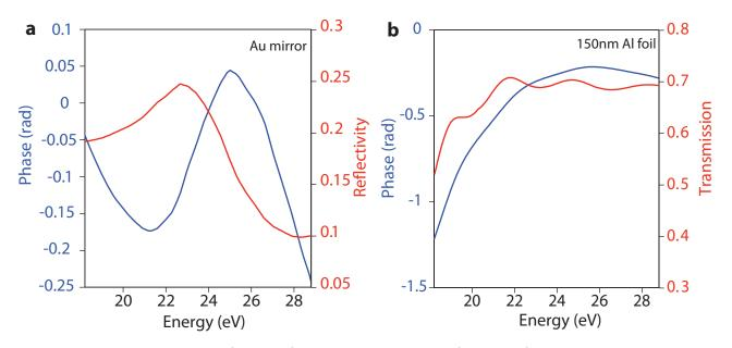
Figure A.1: **a**, Reflectivity (red line) and spectral phase (blue line) of Au coated EUV mirror. **b**, Transmission (red line) and spectral phase (blue line) of 150 nm thick Al foil.
