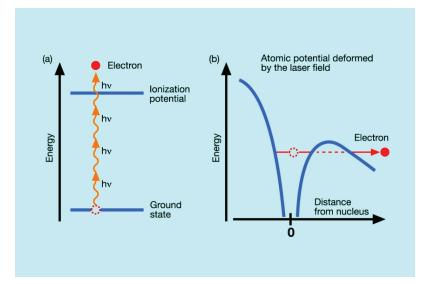
Figure 1.1: Ionization of atoms: transition of electrons from their bound states to continuum in presence of ultrashort laser pulses can occur either by a **a**, multiphoton absorption process or by **b**, tunnel ionization. This figure is adapted from http://wof-cluster.desy.de/.
