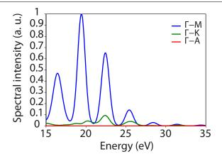
Figure 3.4: Spectra calculated by intraband motion of electrons in the first conduction band of  $SiO_2$  along three different directions of Bouillon zone driven by a 1.5 cycle optical pulse. This figure has been adapted from [23].
