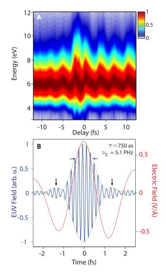
Figure 4.23: **a**, Attosecond streaking spectrogram measured with EUV pulses generated by a  $\sim 1.5$  cycle long optical driver waveform. **b**, Retrieved attosecond pulse after the convergence of PCGPA. Black arrows mark the formation of weak satellite bursts.
