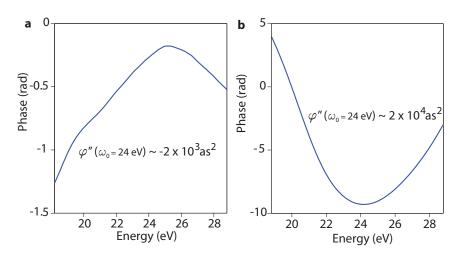
Figure C.1: **a**, Combined spectral phase of a 150nm Al foil and an Au coated EUV mirror. **b**, Calculated spectral phase of the interband contribution to EUV generation from our SBE quantum mechanical simulations.
