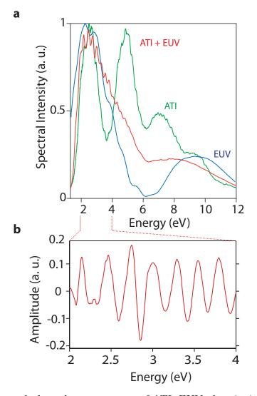
Figure 5.2: **a**, Measured photoelectron spectra of ATI, EUV photoionization and their interference. **b**, Interference fringes of EUV and ATI photoelectrons can be better visualised by removing the DC component in the interference spectrum as presented in **a**.
