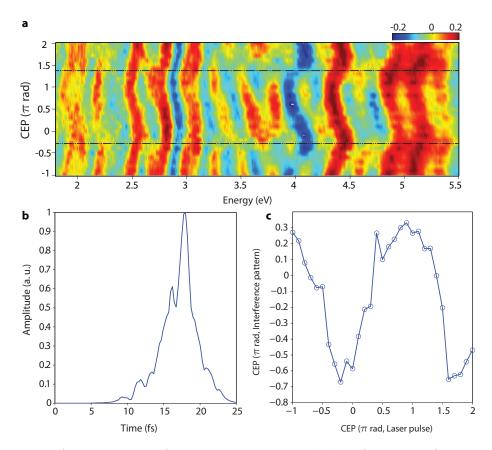
Figure 5.10: **a**, ATI-EUV interference spectra recorded as function of varying CEP of driving laser pulse. **b**, FT of one of the measured interference spectra. **c**, CEP variation of the interference spectra as a function of the varying CEP of driving laser pulse.
