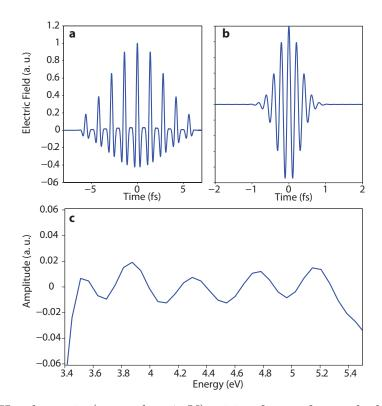
Figure 5.6: **a**, ATI pulse train (centred at 4 eV) arising from a few cycle driving laser pulse. **b**, Isolated attosecond pulse arising from SiO<sub>2</sub>. **c**, Spectral interference between the two pulses at a delay of  $\sim 2$  fs.
