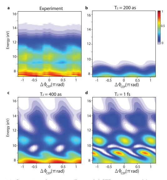
Figure 6.2: Comparison of experimentally recorded CEP spectrogram (**a**) measured with optical attosecond pulses of peak intensity 4 X  $10^{13}W/cm^2$  with the ones simulated by SBEs for three different dephasing times (**b**, **c**, **d**) of the interband polarization.
