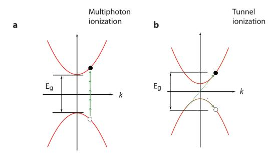
Figure 1.2: Ionization of semiconductors: transition of electrons from valence to the conduction band in presence of ultrashort laser pulses can occur either by a **a**, multiphoton absorption process or by **b**, tunnel ionization, tunnel ionization of electrons in solids is also known as Zener tunnelling. Electrons are represented with black circles whereas holes with white circles. This figure is adapted from Tamaya *et al.* [29].
