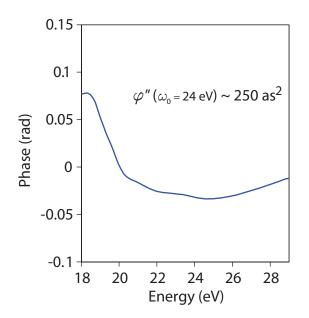
Figure C.2: Spectral phase introduced to EUV pulses in the range 18 - 29 eV by a 20 nm thick SiO<sub>2</sub> nanofilm.
