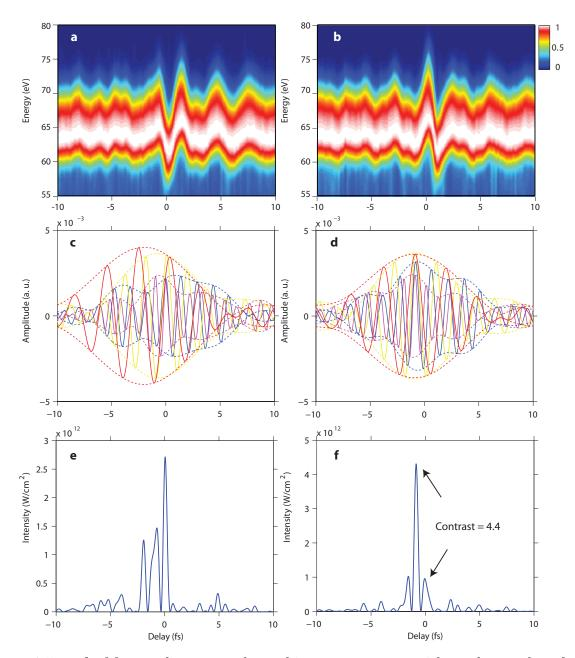
Figure 2.5: **a**, **b**, Measured attosecond streaking spectrograms with random and perfectly synchronised relative temporal phases between individual spectral channels in LFS respectively. **c**, **d**, Reconstructed temporal profiles of individual spectral channels in LFS as retrieved from measured spectrograms in **a** and **b** respectively. **e**, **f**, Reconstructed intensity profiles of electric fields retrieved from streaking spectrograms in **a** and **b** respectively.
