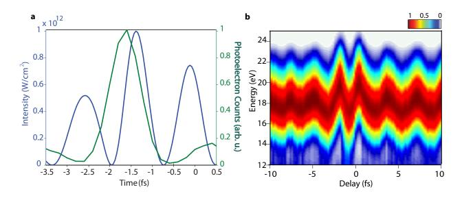
Figure 4.10: **a**, Photoelectron counts (green line) measured as a function of delay between two optical beams as shown in Figure 4.8. **b**, Attosecond streaking spectrogram measured with EUV emission from Ar. Optical driver field intensity (blue line, Figure 4.10a). as retrieved after convergence of PCGPA reconstruction of the experimental spectrogram.
