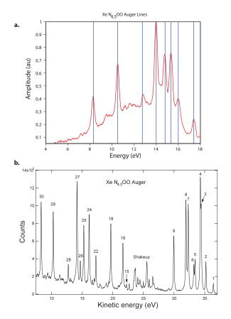
Figure B.1: **a**, Measured photoelectron spectra of Auger electrons excited by EUV photons centred at ~ 95 eV in an ensemble of Xe atoms. **b**, Photoelectron spectra of Auger electrons  $N_{4,5}OO$  of Xe as measured at a synchrotron.
