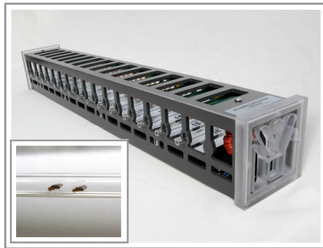
FIGURE 2.6.: Drosophila Activity Monitor. 16 Slots for 5mm diameter glass tubes. Drosophila inside a 5mm diameter glass tubes at the bottom left [4]
