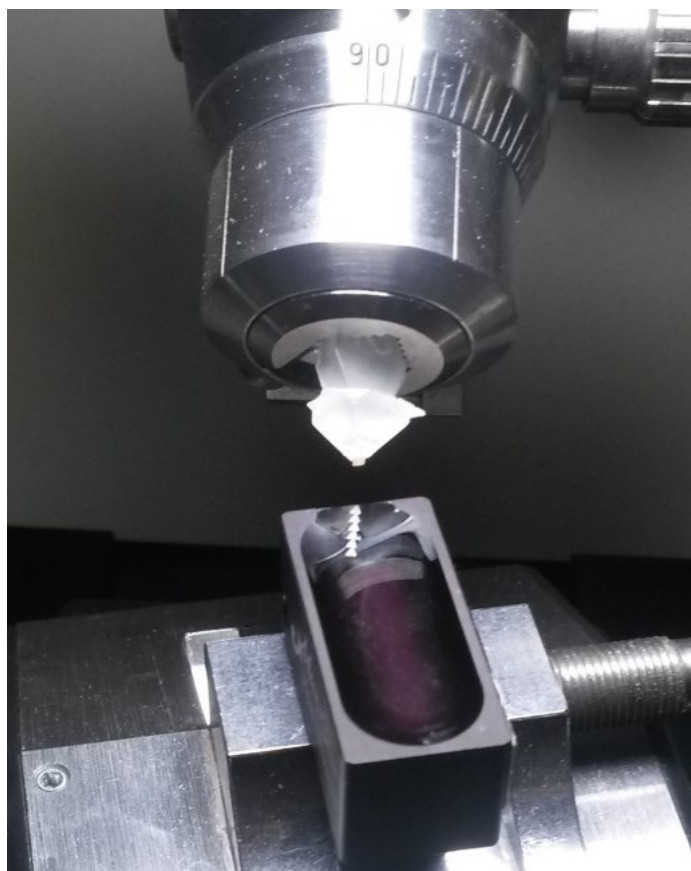
Figure 3.4: The ultramicrotome in action. Shown are the sections of the spirooxazine crystals.
