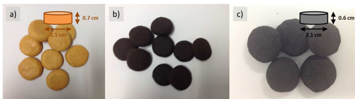
Figure 4 Doughs from glucose–urea–ZnCl 2 /H 2 O + 39% Cellulose before and after baking a ) viscoelastic pellets of the dough, b ) pellets pre-baked at 100°C for 3 hours, the green body, and c ) carbonaceous pellets made at 500°C in nitrogen atmosphere.
