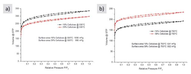
Fig. 5 Nitrogen sorption of carbons made from glucose-urea-salt with different amounts of cellulose (black 16% and red 39%) carbonized at (a) 500 °C and (b) 700 °C in nitrogen after washing.
