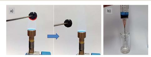
Fig. 6 Images of the nitrogen-doped carbon cookie made from glucose-urea-salt with 39 wt% of cellulose carbonized at 500 °C (a) monolith during repeated firing cycles using a butane/propane gas burner and (b) powder during sorption of methylene blue dye from aqueous solution.
