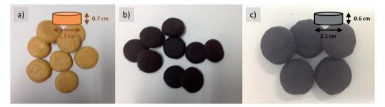
Fig. 4 Doughs obtained from glucose-urea-ZnCl<sub>2</sub>/H<sub>2</sub>O + 39% cellulose before and after baking (a) viscoelastic pellets of the dough, (b) pellets pre-baked at 100  $^{\circ}$ C for 3 hours, the green body, and (c) carbonaceous pellets made at 500  $^{\circ}$ C in nitrogen atmosphere.
