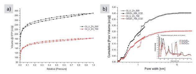
Fig. 3 (a) Nitrogen sorption isotherms and (b) pores size distribution from nitrogen (open circles) and  $CO_2$  (filled circles) sorption of carbons made from glucose, urea, and ZnCl<sub>2</sub> carbonized at 500 °C (black) and 700 °C (red).
