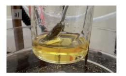
Fig. 1 (a) Liquid monosaccharide-urea melt obtained from glucose.
