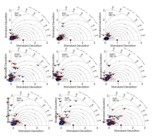
Fig. 3.5.23: Taylor polar plots with daily average standard deviation vs correlation coefficient for three German sites Boltenhagen (54°N), Bamberg (50°N) and Hohenpeissenberg (48°N) for June, July August 2016. O-suite red, control blue.
