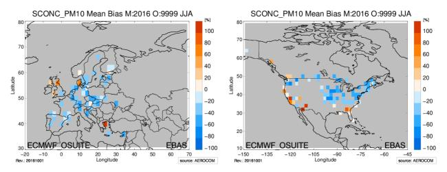
Figure 3.5.1: Bias [%] map of June/July/August mean PM 10 concentrations at EMEP (Europe) and IMPROVE sites (North America); simulated o-suite versus climatological average (2000-2009).
