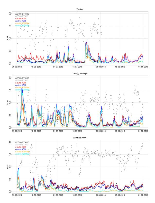
Figure 3.5.7: AOD from AERONET (black dot), AOD o-suite (red line), AOD control (blue line), AOD-Nat o-suite (orange line), AOD-Nat control (cyan line), for the period June 1<sup>st</sup> to August 31<sup>st</sup>, 2016 over Toulon (France), Tunis-Carthage (Tunisia) and Athens (Greece). AOD-Nat corresponds to the natural aerosol optical depth that includes dust and sea-salt.
