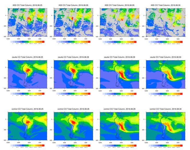
Fig. 5.1.1: CO total column from IASI (top), o-suite (middle) and control runs (bottom) for 25, 26, 29 and 30 of August 2016 over the selected region.
