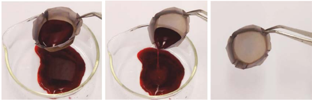
Figure 1.21 Heparinized blood was incubated for 6 h in a superamphiphobic well and removed afterwards by tilting. Macmillan Publishers Ltd., Nature Publishing Group: Nat. Comm. Paven, M., et al., Super liquid-repellent gas membranes for carbon dioxide capture and heart-lung machines, 4, copyright 2013.
