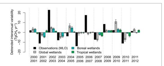
Figure 4. Interannual variability of detrended atmospheric methane concentrations, represented at the atmospheric burden in Tg  $CH_4$ , as measured at the Mauna Loa Observatory (Tg  $CH_4$  yr<sup>-1</sup>), approximately equivalent to the mean global concentrations, and interannual variability in wetland methane emissions for global, boreal, and tropical wetlands. Bars represent the model ensemble mean (n = 11), and the error bars represent one standard error.
