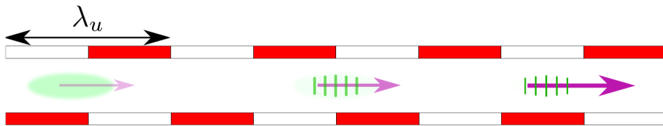
Figure 3: An electron bunch travelling through an undulator is split up into individual microbunches. From Schnorr, 2014, p. 42.
