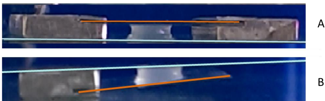
Figure 21 Negative normal force imposed on a fibrin gel polymerized between coverslips separate by two spacer. The top image shows the parallel orientation of the coverslips. Removal of one of the coverslips leads the coverslips moving together imposed by the negative normal force acting on gels polymerized in this geometry (2.1 mm gap size).
