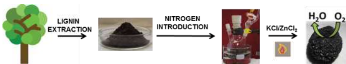
Figure 4.1 Schematic process for the synthesis of mesoporous nitrogen-doped carbon from beech wood lignin.*
