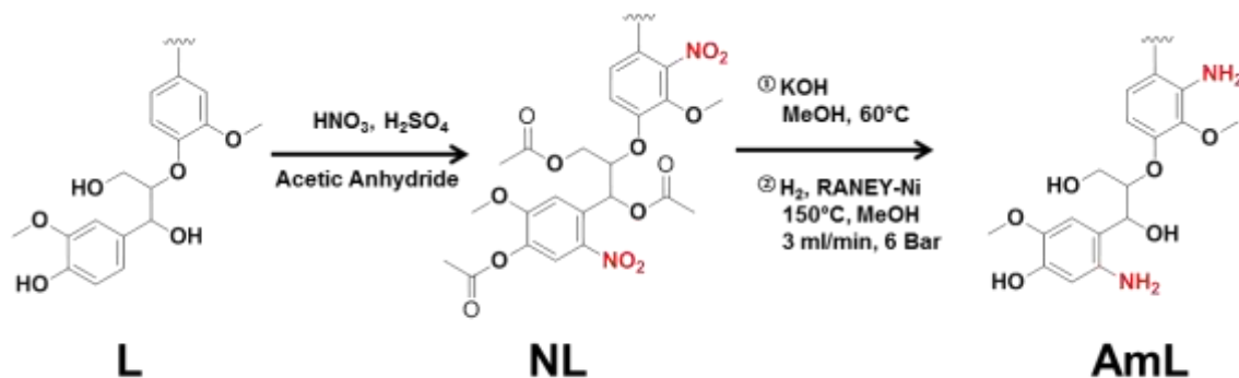
Figure 4.3 Schematic pathway of lignin conversion. From alkali lignin (L) to nitro lignin (NL) via aromatic nitration, followed by reduction of NL to aminated lignin (AmL).*
