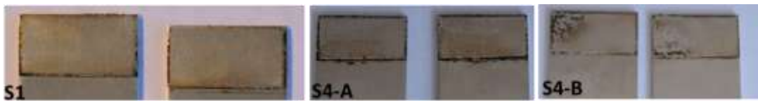
Figure 5.7 Adhesive distribution at the failure after separation of the bars specimens of specimens S1, S4-A and S4-B groups.
