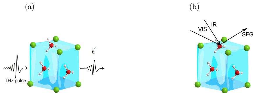
Figure 7.10: Protonic defect transfer: (a) in ice by studying the dielectric complex constant with THz-time domain spectroscopy, and (b) at the ice-air interface by analysing the molecular vibrations of the frozen water molecules. Green atoms represent \text{Cl}^- .
