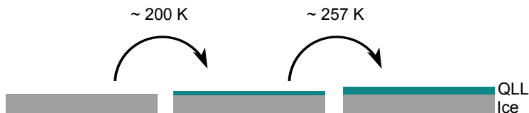
Figure 7.2: Cartoon that summarizes the surface melting of ice: at \sim 200 K a transition from non QLL to a bilayer of QLL was assumed from literature, then at \sim 257 K a transition from one to two QLLs was observed both theoretically and experimentally.
