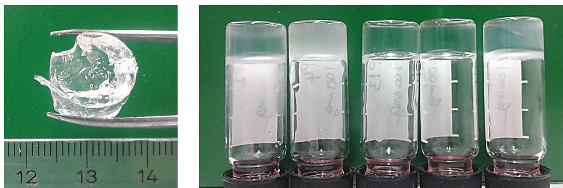
Figure V.9 (a) photo-crosslinked \text{P}(\text{BLG}_{0.84}\text{-CO-LAG}_{0.16})_{171} -dioxane gel ( 100\text{ g}\cdot\text{L}^{-1} ); (b) photo-crosslinked dioxane gels ( 100\text{ g}\cdot\text{L}^{-1} ) of (left to right) \text{P}(\text{BLG}_{0.76}\text{-CO-DLAG}_{0.24})_{59} , \text{P}(\text{BLG}_{0.85}\text{-CO-DLAG}_{0.11})_{53} , \text{P}(\text{BLG}_{0.80}\text{-CO-LAG}_{0.20})_{219} , \text{P}(\text{BLG}_{0.84}\text{-CO-LAG}_{0.16})_{171} , and \text{P}(\text{BLG}_{0.78}\text{-CO-LAG}_{0.22})_{96} .
