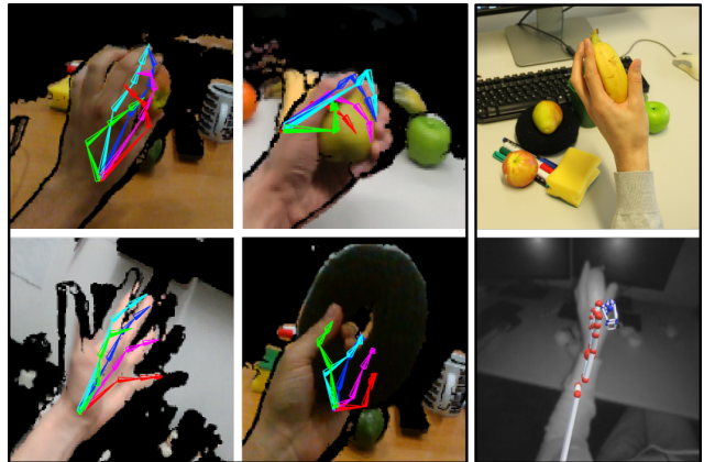
Figure 10: Fast motion that leads to misalignment in the colored depth image or failures in the hand localization step can lead to incorrect predictions (left two columns). LeapMotion Orion also fails under large occlusions (right).
