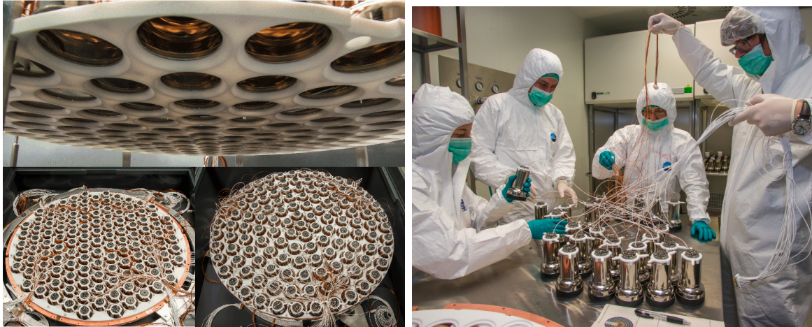
Figure 5.13: (Left) The pictures show the assembled PMT array placed inside the open transport boxes at MPIK. (Right) PMTs are connected to their base and placed inside the array.
