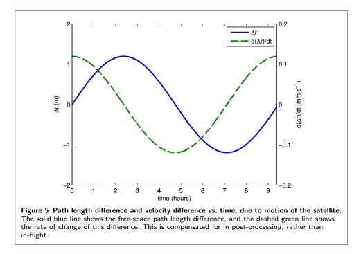
Finally, the radial motion of the satellite causes constant variation in optical path length. To keep the path lengths of the interferometer equal this variation must be continuously compensated for. The time spent in the fibre loop by the part of the photon state in the upper arm, before it is emitted from the satellite, is given by:
