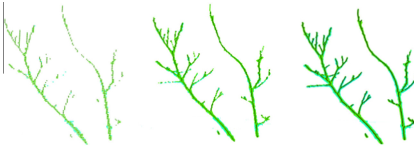
Fig. 9. Laser scanning point clouds obtained for branch arrangements in cube 1 (2 thin branches) for coarse (left), medium (middle), and fine (right) resolution.
