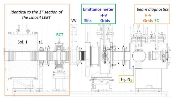
**FIGURE 4.** Layout of the Linac4 H<sup> $\cdot$ </sup> ion source test stand: the first section is identical to the one installed in Linac4 and encompasses a solenoid (sol. 1), horizontal and vertical steerer (s1) and a beam current transformer. After a vacuum valve, the beam diagnostics section contains a slit-grid emittance meter and the Linac4 LEBT beam diagnostics box equipped with grids, a Faraday cup and the injection of the gas mandatory for space charge compensation.
