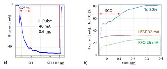
**FIGURE 2.** Linac4 IS03a H<sup>-</sup> operation: a) H<sup>-</sup> current pulse shape, the Linac4 extraction timing (SEJ) is indicated, a 40 mA and 0.6 ms H<sup>-</sup> pulse is shown. b) Transmission of an IS03a H<sup>-</sup> pulse through the RFQ, the pulse's head and tail are chopped in the LEBT. The current before and after the RFQ are measured with beam current transformers. The onset of the Space Charge Compensation (SCC) process is indicated.
