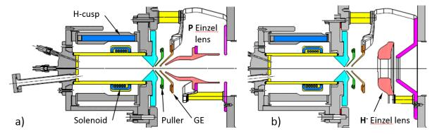
**FIGURE 6.** (a) Layout of IS03p plasma generator and extraction optics. The Halbach offset octupole, RF-solenoid antenna, puller electrode, ground electrode (GE) and Einzel lens are indicated. (b) IS03p plasma generator assembly with its puller and ground electrode mounted on the ion source frontend equipped with the IS03b H<sup>-</sup> Einzel lens.
