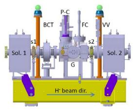
**FIGURE 1.** Scheme of the Linac4 LEBT: the beam current transformer (BCT) is located before the diagnostics box that encompasses the pre-chopper (P-C), horizontal and vertical grids (G) and a Faraday cup (FC). The matching solenoids (sol. 1,2), steerer magnets (s1,s2) and sector valve (VV) are indicated.
