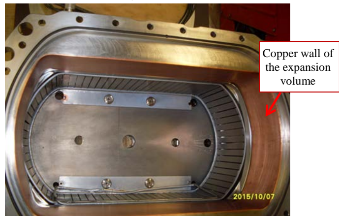
FIGURE 2. View inside the BATMAN source with race-track shaped driver.
