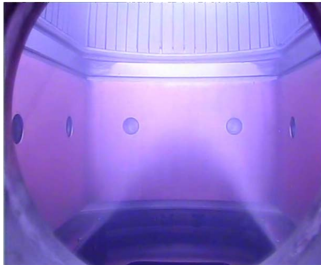
FIGURE 3. Plasma light inside the BATMAN source with racetrack shaped driver.
