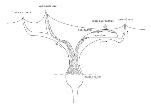
Figure 7 Schematic cross section of the  $CO_2$  hydrothermal systems at Yonaguni Knoll IV hydrothermal site. The dotted line indicates the depth at where boiling starts (adapted from Konno et al. 2006).
