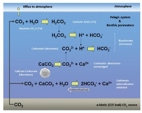
Figure 3 Ocean carbonate system under the influence of CCS leak and the escape of liquid  $CO_2$  (www.bgs.ac.uk/qics).
