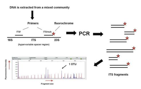
Figure 8 ARISA workflow (Böer 2008). Amplification of DNA produces fluorescently labelled fragments of different length of the ITS region which are detected and separated by capillary electrophoresis.
