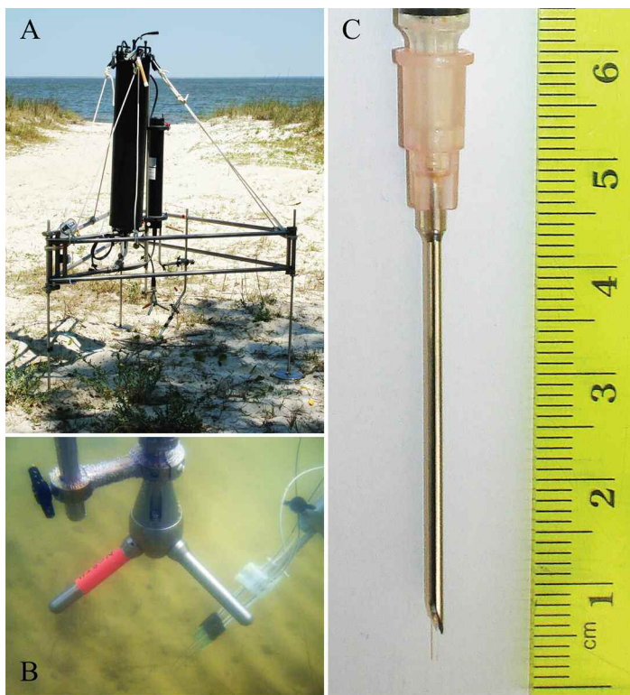
Fig. 1. (A) Eddy correlation instrument with oxygen optode. (B) ADV sensor head and two optodes. (C) Optodes housed in 1 mL syringe. The dark spot at the end of the glass fiber protruding from the needle is the sensing dye. The dark line parallel to fiber is the shadow of the fiber.
