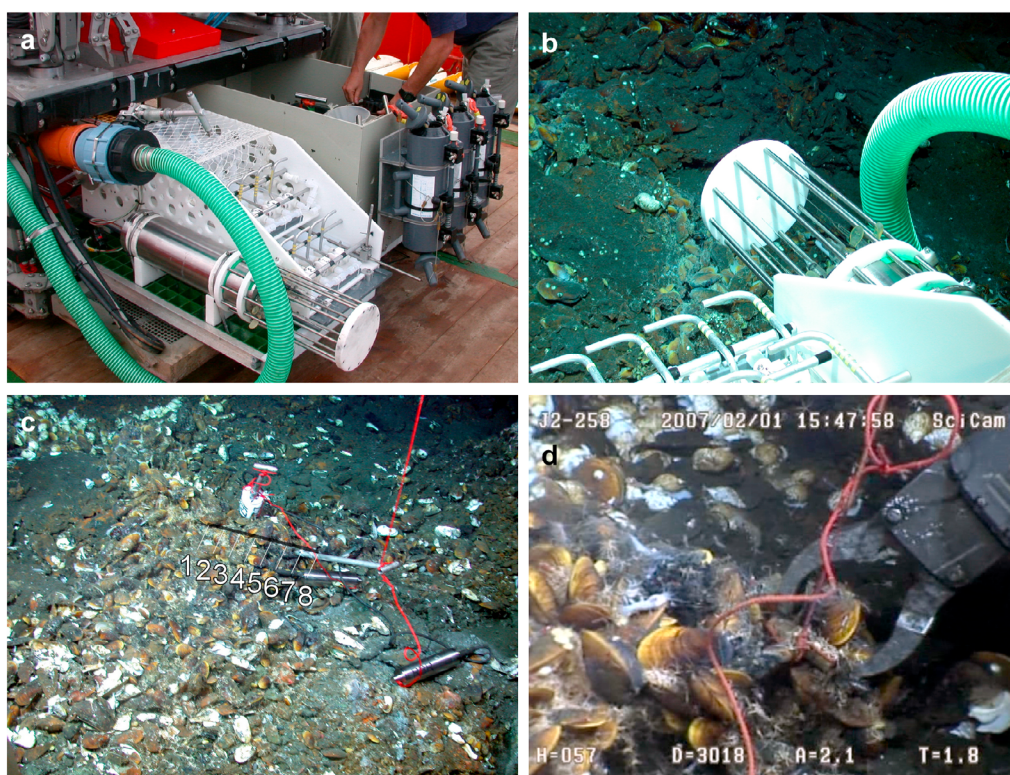
Figure 2. In situ instrument (ISI) and 8-channel temperature lances. (a) ISI setup on the extendable drawer of the ROV Quest (left). (b) ISI taking measurements on above a small mussel patch at Site 4. Copyright, MARUM University of Bremen. (c) T-logger site with two 8-channel temperature lances pushed horizontally (at an angle of about 20°) and vertically into the mussel bed. The black line indicates the position of the horizontal temperature lance within the mussel bed, while 1–8 marks the position of the temperature sensors inside the lance. Copyright, MARUM University of Bremen. (d) Recovery of the horizontal temperature lance. Copyright, Woods Hole Oceanographic Institute.
