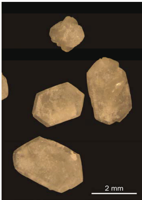
Figure 5: Euhedral, tabular gypsum crystals with a size between 1.5 and 4 mm. Often, the crystals occur as twins.
