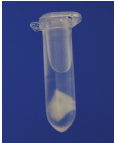
Figure 6. Photograph of the precipitated nucleic acid in an Eppendorf tube after addition of 0.6 vol of cold isopropanol (step 8).
