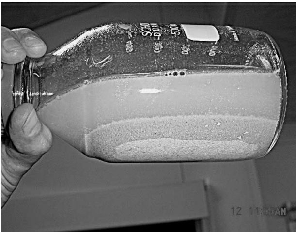
Fig. 9. Sand-size carbonate particles (light deposit in bottle) released after vigorous shaking of Phase 6 mucus aggregates (darker deposit) collected in a bottle
