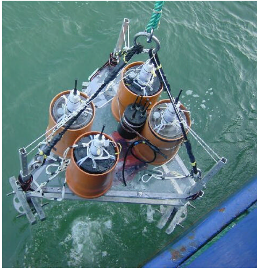
Figure 5: Framework with the motor device and four brackets for the transporting of the experimental chambers. For the incubations, the motor was connected by wires to the single chamber in order to operate the rotating disk.
