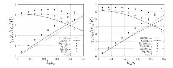
Figure 4. Spectra for  $R/L_{Ti,e} = 12.5, 20$  from left to right respectively. GENE simulations  $\gamma$ : solid curve (×) and  $\omega_r$ : solid curve (+) against results obtained solving Eq. (10) ( $\gamma$ : filled dots and  $\omega_r$ : stars) and Eq. (9) ( $\gamma$ : open dots and  $\omega_r$ : triangles) are presented. The dashed line represents the  $\omega_{*pi}/2$  frequency.
