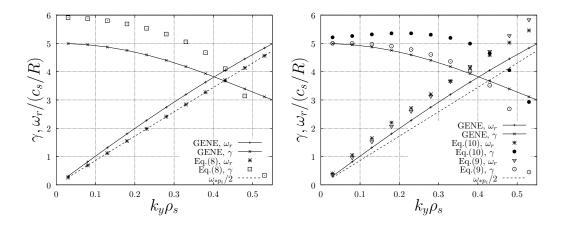
Figure 3. Spectra for  $R/L_{Ti,e} = 15$ . On the left GENE simulations  $\gamma$ : solid curve (×) and  $\omega_r$ : solid curve (+) against results obtained solving Eq. (8) ( $\gamma$ : squares and  $\omega_r$ : stars) are presented. On the right results obtained solving Eq. (10) ( $\gamma$ : filled dots and  $\omega_r$ : stars) and Eq. (9) ( $\gamma$ : open dots and  $\omega_r$ : triangles) are presented. The dashed line represents the  $\omega_{*pi}/2$  frequency.
