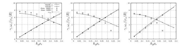
Figure 2. Spectra for  $R/L_{Ti,e} = 35, 40, 45$  from left to right respectively. On the plot GENE simulations  $\gamma$ : solid curve (×) and  $\omega_r$ : solid curve (+) against results obtained solving Eq. (8) ( $\gamma$ : squares and  $\omega_r$ : stars) are presented. The dashed line represents the  $\omega_{*pi}/2$  frequency.
