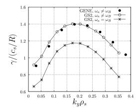
Figure 6. KBM spectra for  $R/L_T = 6.89$ ,  $\beta=1.5\%$  1) GENE,  $\omega_{\kappa} \neq \omega_B$ , filled circles; 2) GS2,  $\omega_{\kappa} \neq \omega_B$ , open circles; 3) GS2,  $\omega_{\kappa} = \omega_B$ , stars.
