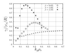
Figure 1. A typical transition of the spectrum of microinstabilities in a local flux tube simulation. From electrostatic ITG ( $\beta = 0\%$ ) to KBM ( $\beta = 1.5\%$ ). Here  $\gamma$  is the growth rate,  $k_y \rho_s$  the mode wavelength, with  $\rho_s$  the sound ion Larmor radius.
