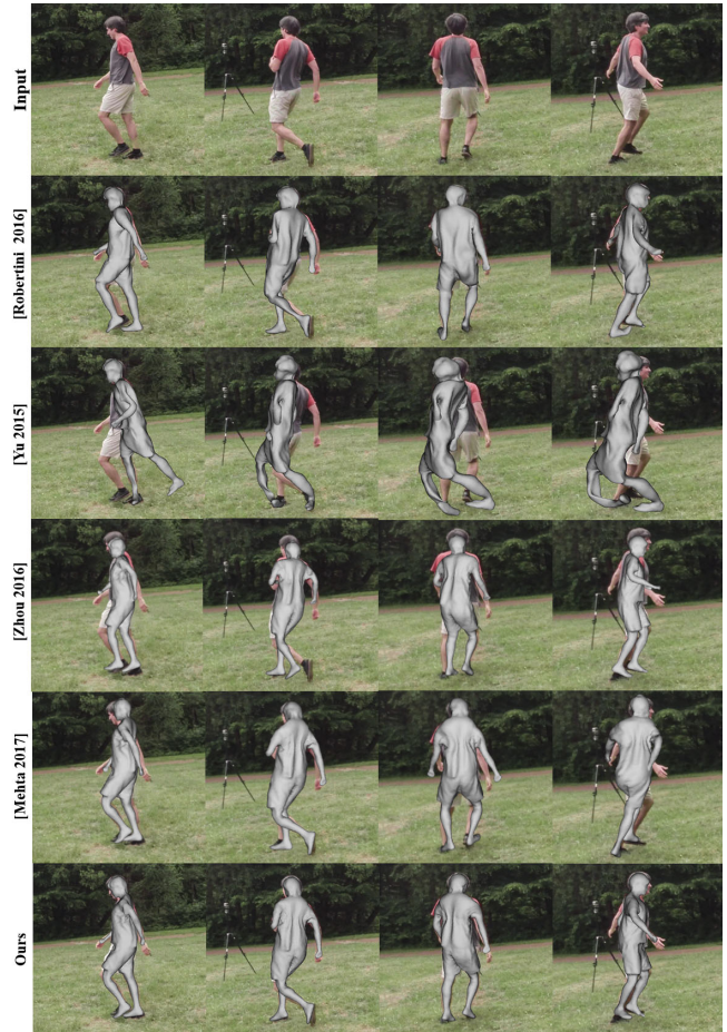
Fig. 11. Qualitative shape comparison on the Pablo sequence. Our approach obtains comparable quality as the multi-view approach of [Robertini et al. 2016] (8 cameras) and drastically outperforms the template-based monocular tracking approach of [Yu et al. 2015]. In comparison to rigging the template model with respect to the 3D pose estimation results of [Mehta et al. 2017] and [Zhou et al. 2016b], our approach yield more accurate results with less artifacts that better overlay with the input.
