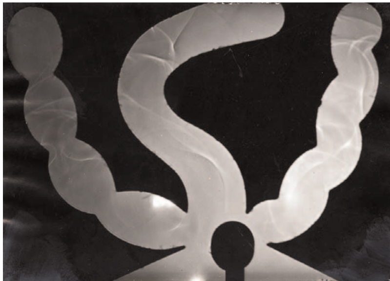
Figure 17 Franz Max Osswald, sound test in a model of the Ear of Dionysius, a Sicilian cave that is surrounded by a myth of perfect sound conductivity, 1930 (Image Archive, ETH Library Zurich, http://doi.org/10.3932/ethz-a-00098644 ).
