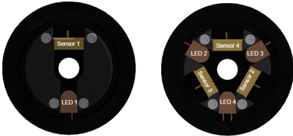
Figure 3.14: Light barrier arrays. Left: first diode chamber. Right: Second diode chamber [Ale11]
