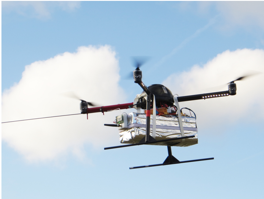
Figure S10: COCAP mounted under a custom-built multicopter (Sensomotion UG, Germany and Ostwestfalen-Lippe University of Applied Sciences, Germany)
