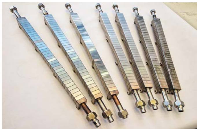
Fig. 1 The image shows the WEST divertor PFUs prototypes. Six of them were HHF tested in GLADIS. Each of them are about 0.6 m long PFU and made of 35 W monoblocks bonded on a CuCrZr cooling tube with \varnothing 12 mm inner diameter equipped with a swirl as turbulence promoter.
