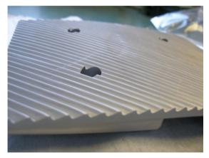
**Fig. 6.** Reflector #8, machined from graphite with optimized grating and coated with tungsten.
