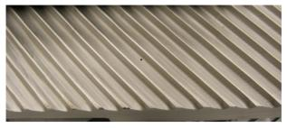
Fig. 8. Flush mounted NiCr-Ni thermocouple, its tip can be recognized as a small bright spot within the borehole. The borehole diameter of 0.5 mm is already in cutoff for the millimetre wave.
