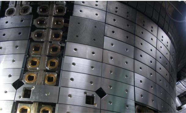
**Fig. 9.** Top: Grooves machined into the rear part increase the shielding of the thermocouples and their cables. In addition, cables are protected by flexible stainless steel tube. Bottom: Reflector #8 assembly completed inside AUG.
