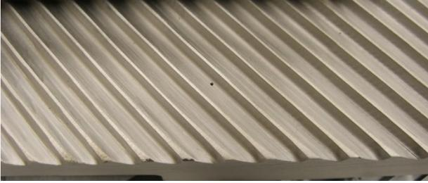
**Fig. 8.** Flush mounted NiCr-Ni thermocouple, its tip can be recognized as a small bright spot within the borehole. The borehole diameter of 0.5 mm is already in cutoff for the millimetre wave.
