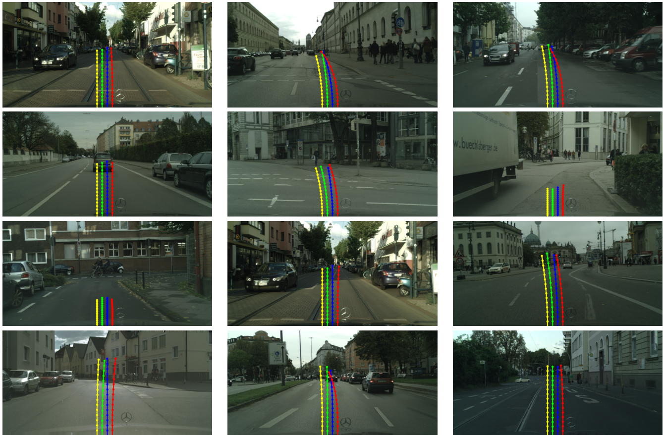
Figure 6: Odometry prediction: We show predicted odometry for 15 time-steps as points (bottom to top) over-layed on the last visual observation. The distance and angle between subsequent points is the predicted (proportional) speed and steering angle. Color codes: Blue : Ground-truth, Red : Kalman Filter, Yellow : Our LSTM without visual input, Green : Our LSTM with visual input.
