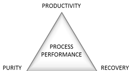
Figure 4.1. Trade-off between productivity, purity and recovery to provide the optimal process performance.
