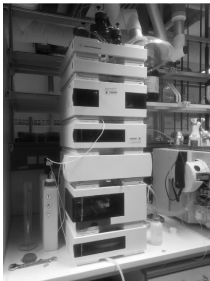
Figure 6.1. HPLC unit used for separation of bicalutamide enantiomers.
