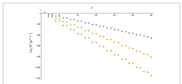
**Figure A4.** The figure illustrates the value of  $\log \|\mathbf{f}'(\mathbf{p}^{\infty})^n\|$  as a function of successful distillation rounds for single qubit white noise  $10^{-2}$  (blue),  $10^{-3}$  (yellow) and  $10^{-4}$  (green).
