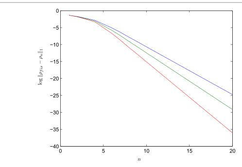
**Figure A1.** The figure illustrates  $\log \|\rho_{\text{fix}} - \rho_n\|_1$  for different noise parameters f = 0.97 (blue), f = 0.98 (green) and f = 0.99 (red). The fixed point  $\rho_{\text{fix}}$  was evaluated for 500 iterations of the DEJMPS protocol.
