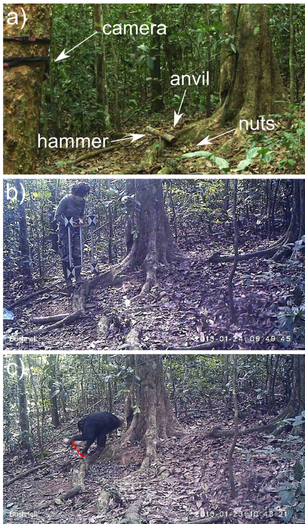
Fig. 1 a A typical lab-site: a camera trap attached to a tree trunk, with an open view of a root anvil with an experimental hammer and nuts. b GS is videotaping the calibration device, orienting it in different positions; this picture shows the orientation selected as the best approximation of the plane along which the hammer-lifting movement occurred in (c). c The red dots show the position of the hammer at each frame, during the lifting movement. The composite figure was created in Inkscape 0.91
