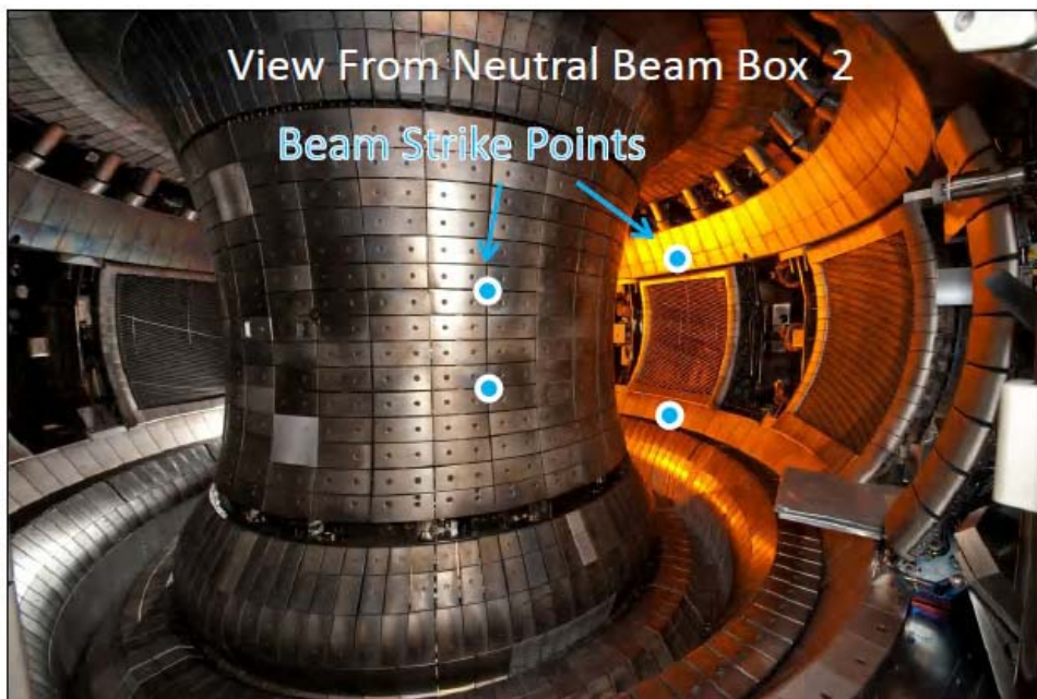
Figure 1.7.: The approximate radial and tangential shine through location as viewed from the neutral beam box 2.
