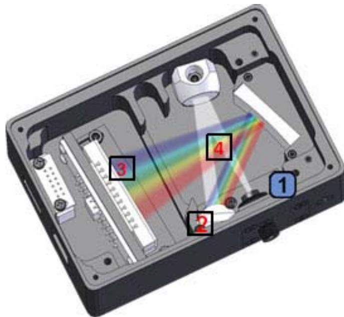
Figure 2.8.: Illustration of the working principle of an IR spectrometer [20]. 1 = slit 2 = grating 3 = detector 4 = optical bench
