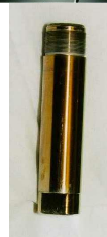
sample holder L = 70 mm Ø = 15 mm
