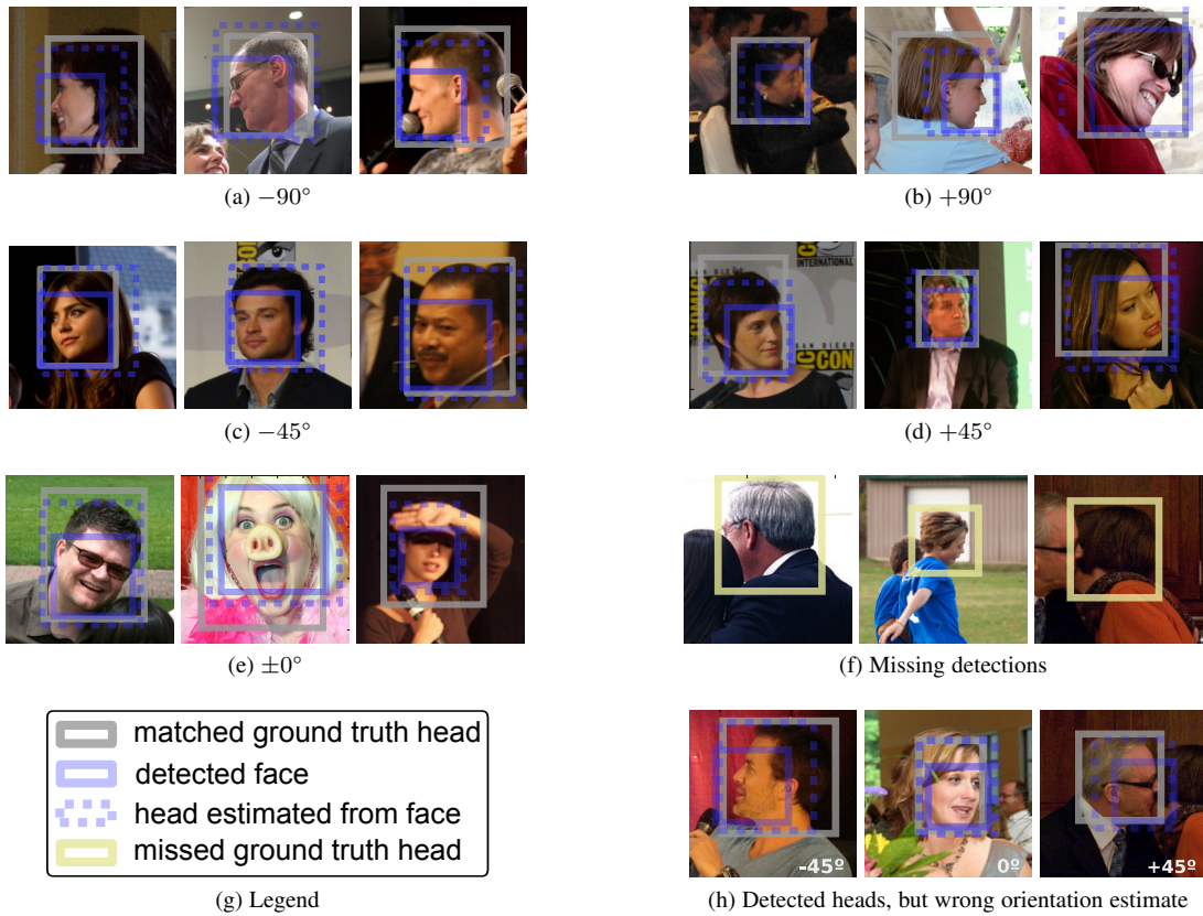
Fig. 19: Example results from the face detector (PIPA val set), and estimated head boxes.
